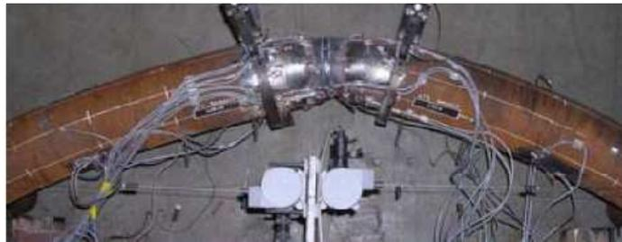
**FIG. 1.4:** Local buckle in an instrumented length of pipe, after Carr *et al.* [7].
