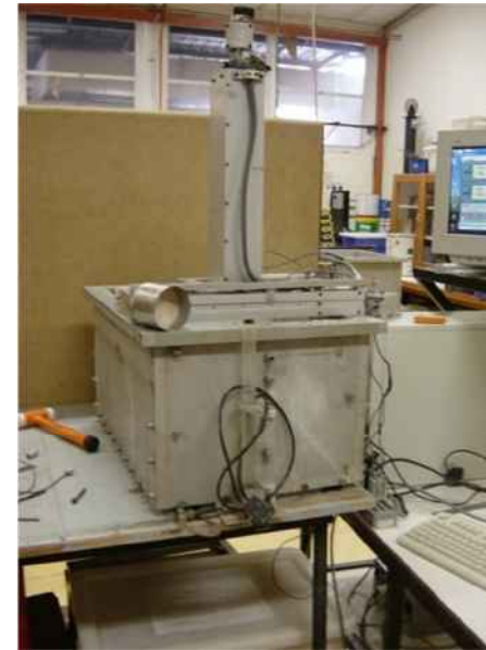
Figure 7.2.3. Close-up photograph of the actuator used in the UWA centrifuge.
