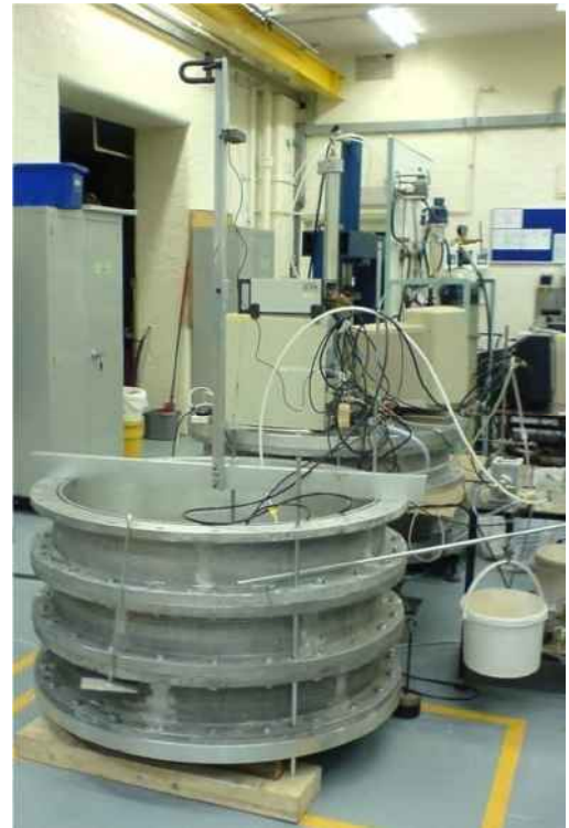
Figure 4.1.8. Installation apparatus used for layered soil tests.
