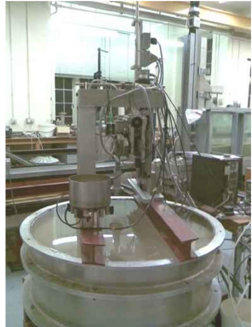
Figure 6.2.3. Photograph showing the layout of the 3DOF rig and tank for the caisson grouting experiments. The caisson is shown in the picture placed on its lid to protect the skirt.
