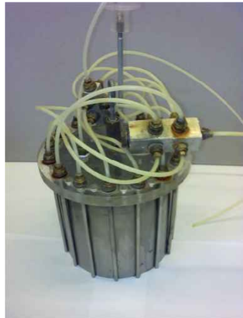
Figure 4.3.10. Photograph of Caisson 4 with the injection apparatus attached. The system could be configured to allow alternate injection and pressure measurement.
