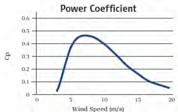
Figure 1.2.6. The variation of wind turbine power coefficient with wind speed for a Vestas 1.65 MW wind turbine. The trend of the curve is typical for commercially available wind turbines. (Vestas (2008a))
